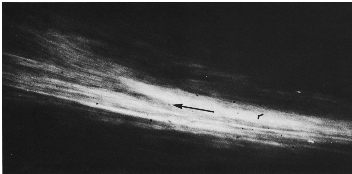
Fig.2. Optical micrograph taken between crossed-polarisers of a sample of actin paracrystals (0.5 mg/ml, 50 mM KCl, 25 mM \text{MgCl}_2 ) formed in a magnetic field of 10 T. The arrow shows the field direction. Magnification \times 100 .
